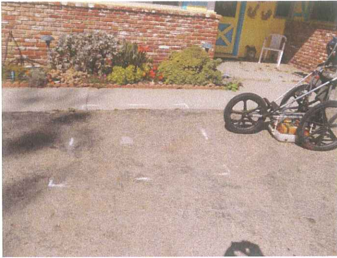
Fig. 1 - Photo and saved GPR file of a possible buried septic tank confirmed on the east side of the of the existing house property.
